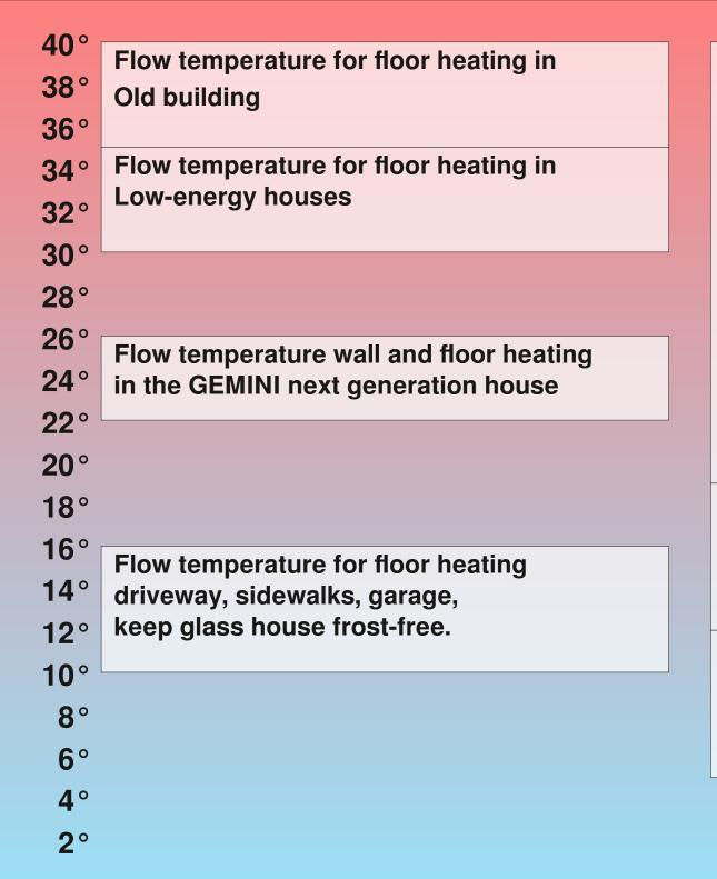
Maximum extended temperature range of the low-temperature heat storage.
